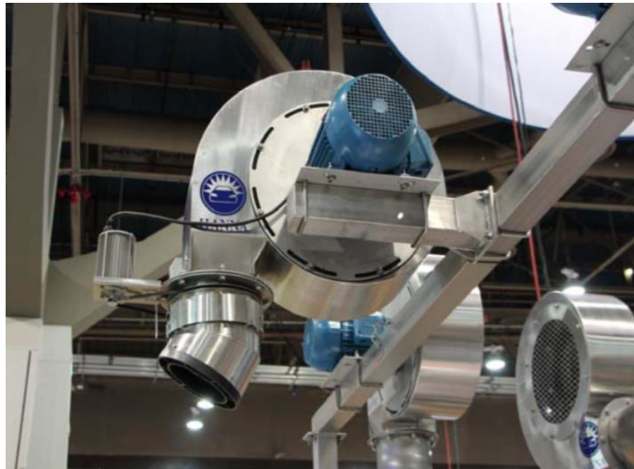
Five motor configuration utilizing (H815406) Blower Support Bracket for center blower
